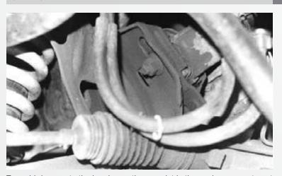
To avoid damage to the header coating or paint in the engine compartment it may be necessary to raise the right side of the engine while installing the passenger side BBK Header. The motor mount is connected to the vehicle with 1 nut, easily accessible from under the front of the vehicle.
